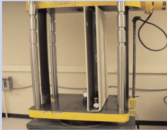
Figure 3: Typical specimen with sheathing.
