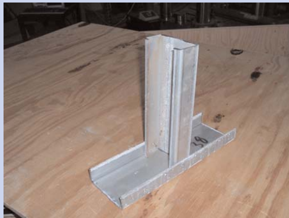
Figure 4: Typical stub column test specimen without sheathing.
